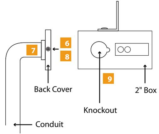
**7** Remove the knock out and mount the conduit.
