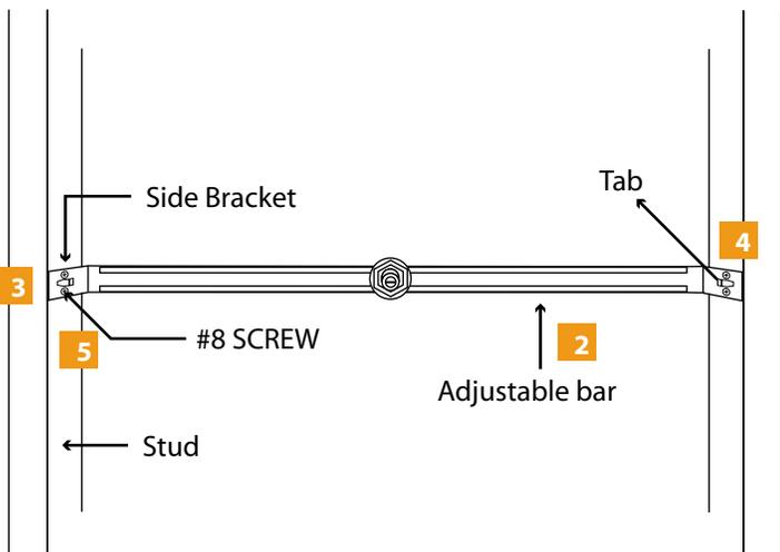
**2** Place the adjustable bar between the studs.
